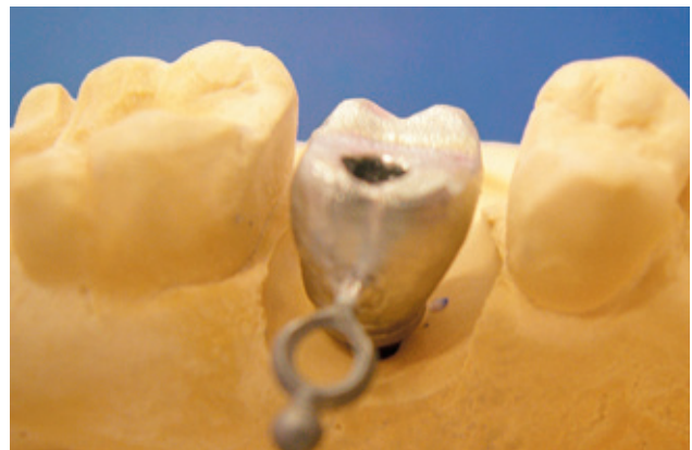
Fig 8 Cast titanium structure onto abutment without pre-welding, palatal view.
